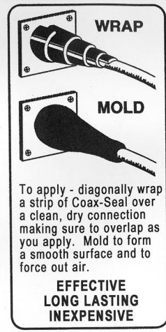
To apply - diagonally wrap a strip of Coax-Seal over a clean, dry connection making sure to overlap as you apply. Mold to form a smooth surface and to force out air.
